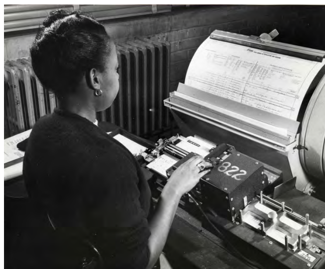
A 1950 census worker creating a punch card to tabulate census data, Library of Congress.
